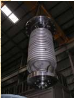
Seal Cooler for a Nuclear Plant Pump
