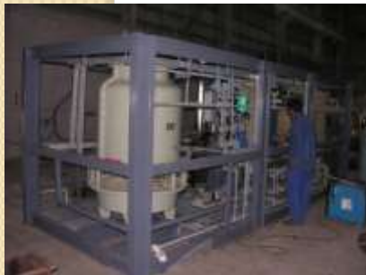
Skid Mounted Solar Cooling System for an experimental R&D Project in Australia
