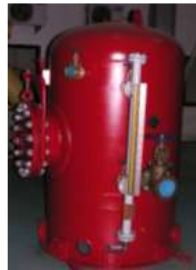
Rubber lined vessel for an FPSO
