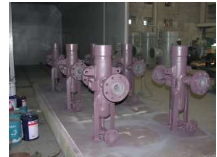
Strainers emerging from Shot Blast Chamber
