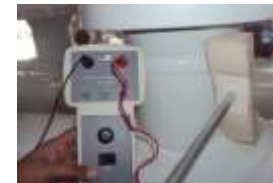
Holiday Test of protective non-conductive coating on metallic surface
