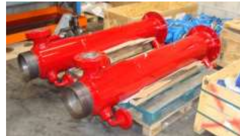
Upstream wellhead Liquid Filter – Working Pressure 10000 psig in special construction AISI 4130
