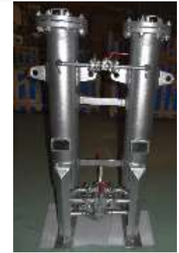
Duplex Filters for a compressor station
