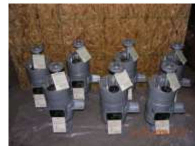
Automatic Air Vents ( AV125 / AV150)
